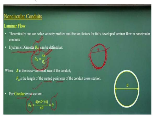
But when you go for a noncircular case you need to define as a equivalent flow okay. So that means we introduce a hydraulic diameters okay, it is called as hydraulic diameters,
