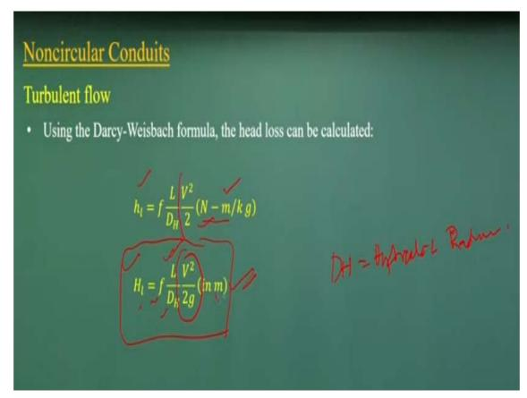
The head loss is a functions of the velocity head which is
