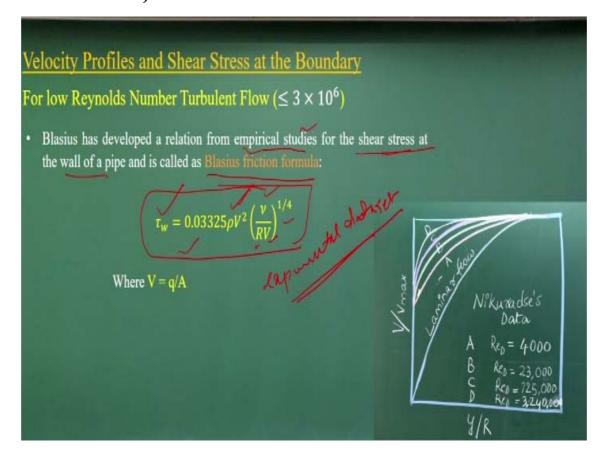
But when you look it what could be the shear stress that is what is the wall shear stress, shear stress at the wall of the pipe. That is what is also empirically established with the functions of wall stress, the average velocities and hydraulic radius and V. That is what is develop it to compute it what could be the wall stress from experimental data set, from experimental data set it derive.
