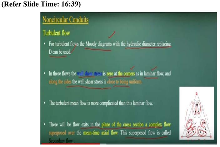
Now if you look it that if you have the turbulent flow same case you have a turbulent flow the velocity distributions as well as the wall shear stress distributions exchanges it. What we do it in any case of the turbulent flow we also use the Moody's diagrams. Hydraulic diameters replacing with a D. That is what is used to quantify what could be the energy losses.
