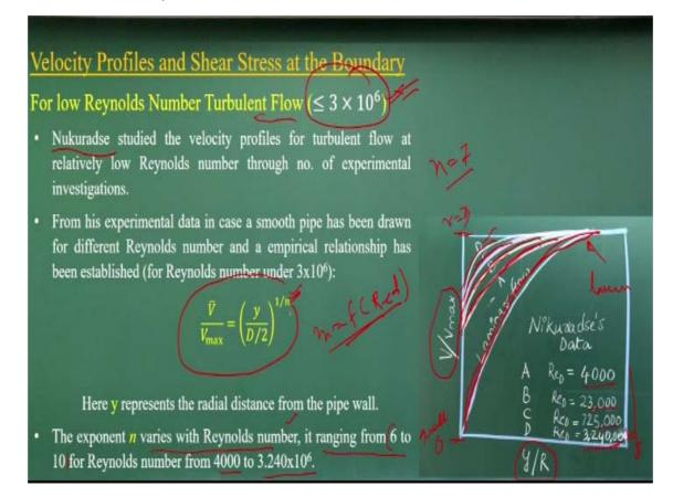
Now coming back to the velocity profile, or the shear stress at the boundary. Here we divide into two zones as suggested by Nikuradse by conducting a series of experiment, finding out velocity profiles for the turbulent flow where you have the flow Reynolds number less than three millions okay. If you look at this Reynolds numbers, okay it is too large okay.
